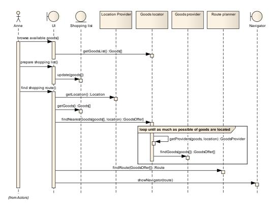
Figure 2 Sequence diagram for the main shopping activity scenario
